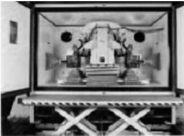
Figure 5.14. Combined testing system: vibration, climate, and corrosion [148].
