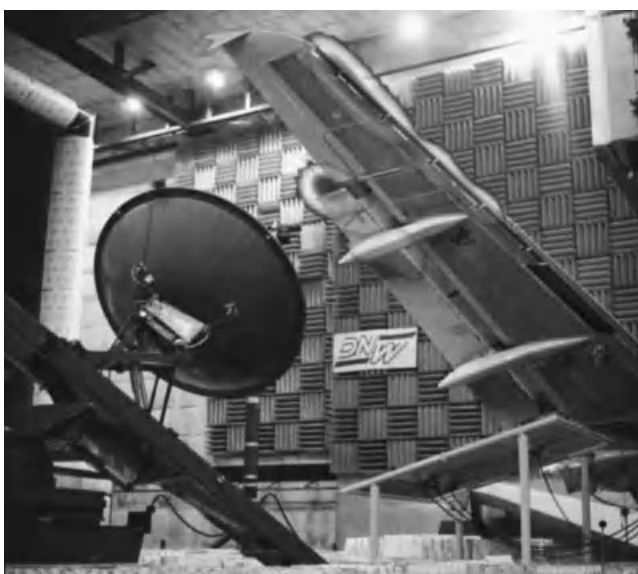
Figure 5.58. Acoustic measurements on a full-scale wing of the Airbus A320 in the open jet test section of the DNW-LLF.
