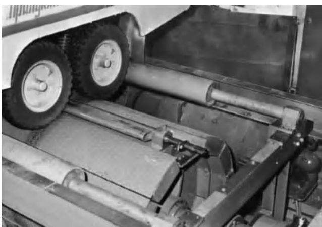
Figure 5.36. Working heads of vibration equipment with test subject (car's trailer).
