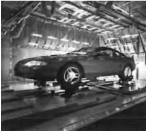
Figure 5.65. Sample drive-in chamber for full vehicle testing (Cincinnati Sub-Zero).
