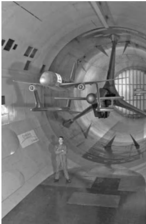
Figure 5.59. The test section of the wind tunnel ONERA—The French Aerospace Lab [175].
