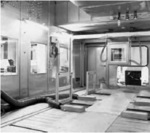
Figure 5.15. Climate test chamber combined with dynamometer [148].
