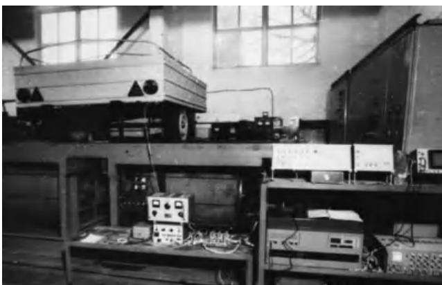
Figure 5.35. Equipment for vibration testing with test subject—a car's trailer (from backside).
