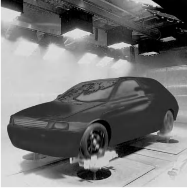
Figure 5.53. Cold heat climate test chamber with a four-poster system and sunlight simulation [148].
