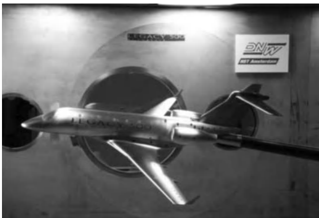
Figure 5.57. Force and pressure measurements on a model of the Embraer Legacy 500 in the transonic wind tunnel DNW-HST.
