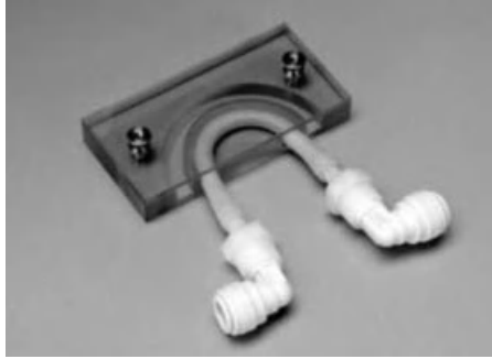
Figure 1.7. Bose fixed bend fixture for stent fatigue testing [25].
