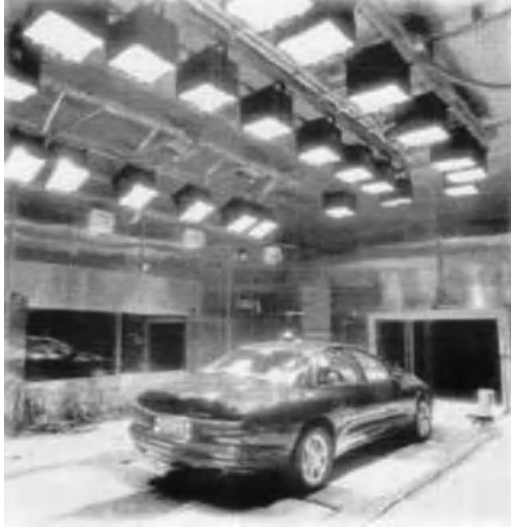
Figure 5.64. Large solar simulation system for testing automobiles and other products [40] (Atlas Material Testing Technology [MTT] LLC).
