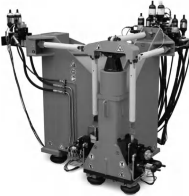
Figure 5.31. MTS Multiaxial Elastomer Test System—Model 836 [157].
