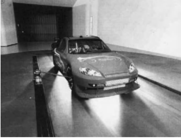
Figure 5.11. Climate test chamber on rolling roads (MTS Systems Corporation) for the whole product (Windshear Inc.).
