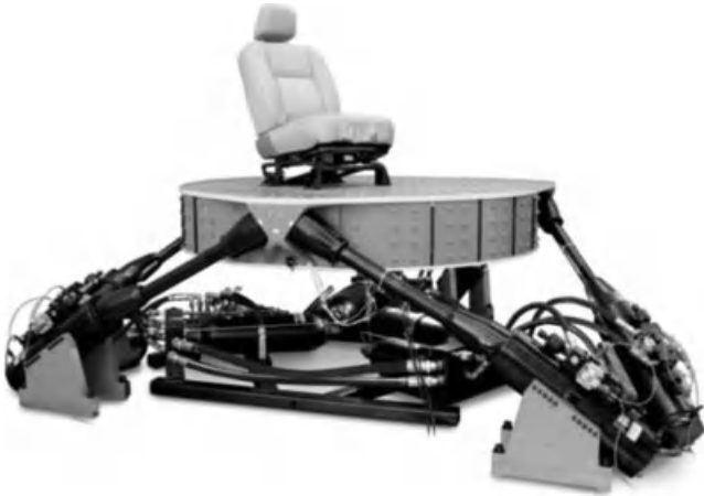
Figure 5.30. MTS Model 353.20 Multi-Axial Simulation Table (MAST) for vibration testing [155].
