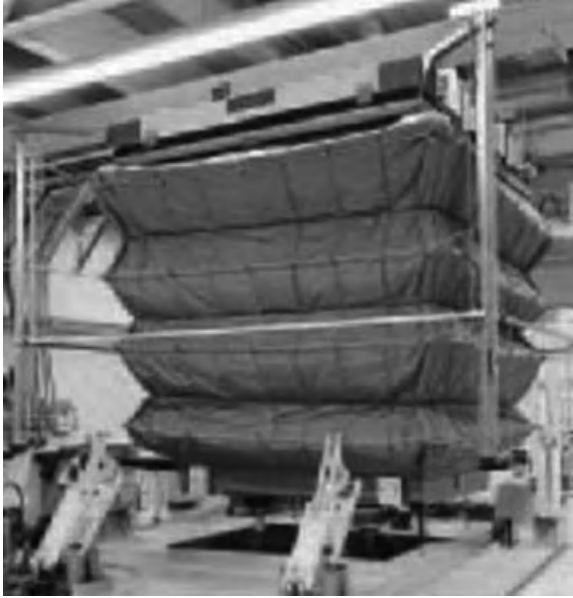
Figure 5.13. Cold-heat climate test chamber with multiaxis vibration table [148].
