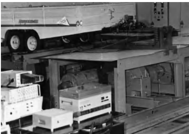
Figure 5.34. Equipment for vibration testing with test subject—car's trailer (from front-back side).
