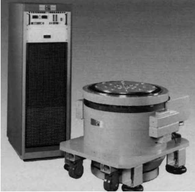
Figure 5.28. R-Series electrodynamic vibration equipment produced by Unholtz-Dickie Corporation [154].
