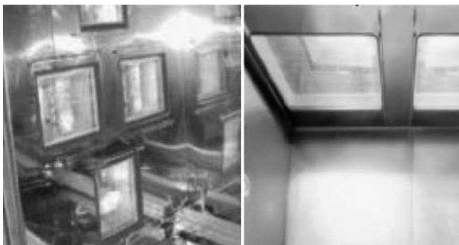
Figure 5.63. Inside components of test chamber Atlas Material Testing Technology (MTT) SC2000 [178].
