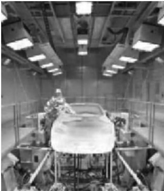
Figure 5.12. Cold-heat climate test chamber with road simulator and sunlight simulator [148].
