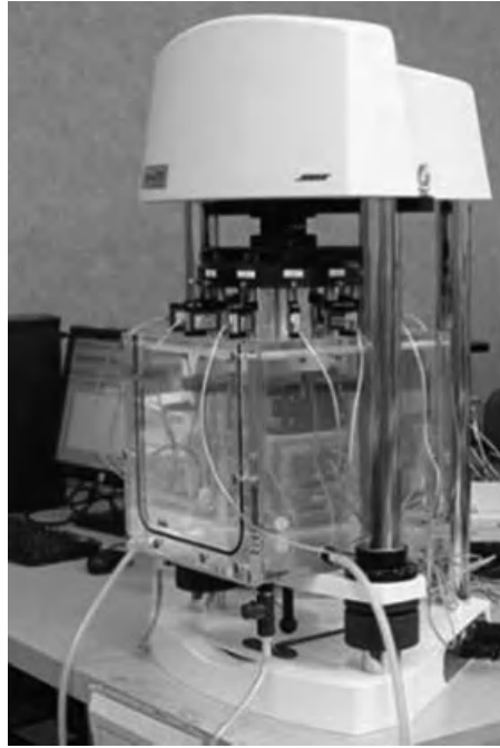
Figure 1.6. ElectroForce® multiple-specimen stent durability testing system [30].
