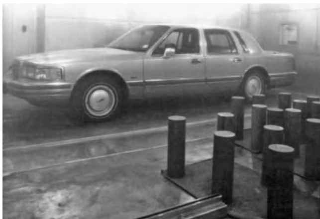
Figure 5.48. High-performance Thermotron chamber for automotive industry to test vehicles under extreme temperature and humidity conditions.
