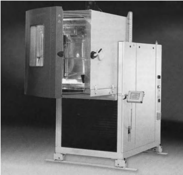
Figure 5.17. Combined test chamber with vibration equipment [148].
