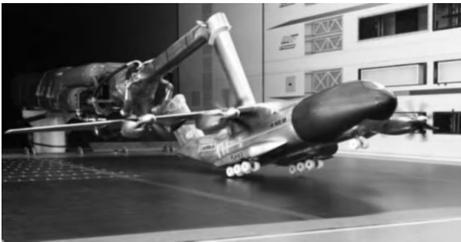
Figure 5.56. Engine and ground simulation tests on a model of the Airbus A400M above a moving belt in the 8 \times 6 m test section of the DNW-LLF.
