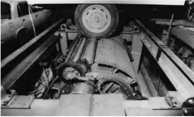
Figure 5.37. Working heads of vibration equipment with wheel of the car's trailer.
